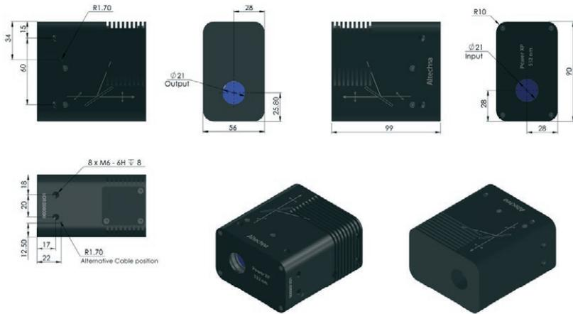
Figure 13. Main dimensions and mounting options of PowerXP.
