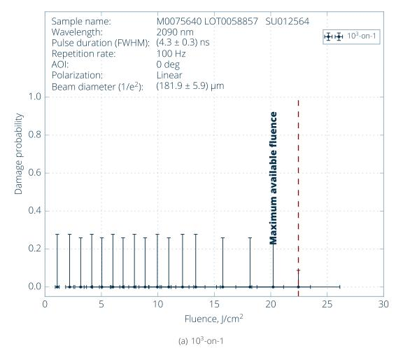
Figure 2. Damage probability plot.
