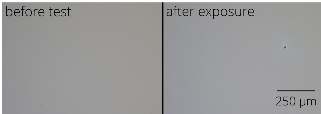
Figure 5. Typical damage morphology: fluence 12.1 \text{ J/cm}^2 , damage after 28 pulse(s).
